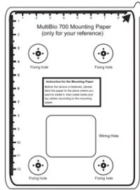
(1) Post the mounting template on the wall. Drill the holes according to the marks on the template (holes for screw and wiring).
