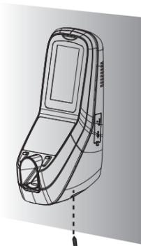
(5) Fix the device to the back plate.
