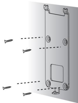
(4) Fix the back plate on the wall according to the mounting paper.
